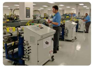
Developing optimized sealing solutions requires sophisticated testing and analytical methodology, thus SKF operates a global network of dedicated testing facilities. Every year, these state-of-the-art laboratories conduct thousands of tests, including durability, performance, contaminant exclusion, salt fog corrosion, cold fracture, pump rate, friction torque, dry wear, and chemical compatibility.
